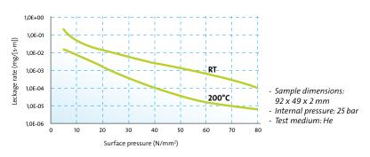
novatec® PREMIUM XP is designed for minimum leakage. The microporosity of the innovative gasket material decreases under the influence of temperature and surface pressure.
