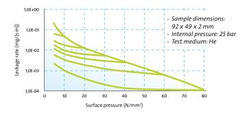
The new generation of novatec® PREMIUM XP demonstrates considerably less leakage at the standard surface pressure levels.
