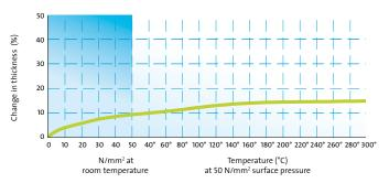
The thickness of novatec® PREMIUM XP decreases to a particularly small extent under the influence of temperature. At 300°C, thickness is only 5 % lower than at room temperature.
