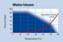
The pressure and temperature limits indicated are influenced to a major extent not only by the characteristics of the material but also by the installation conditions (the surface pressure level in particular). The information provided must therefore be considered an estimate that is on the safe side rather than a fixed application limit.
