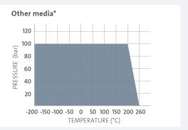
The temperature and pressure recommendations in the graphs apply to gaskets 2.0 mm thick that are used with raised face flanges. Higher stresses are possible when thinner gaskets are used! The information provided must therefore be considered as estimates that are on the safe side rather than as specific operational limits.
